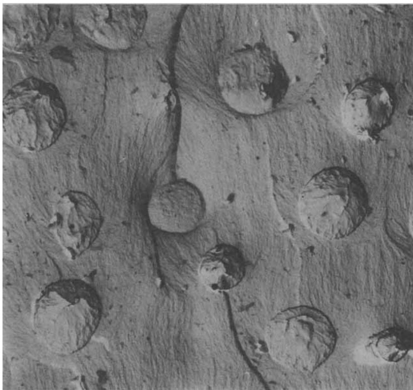
FIGURE 1 Replica transmission electron micrograph of fracture surface of rubber-modified epoxy material. Magnification \times 7500 .
